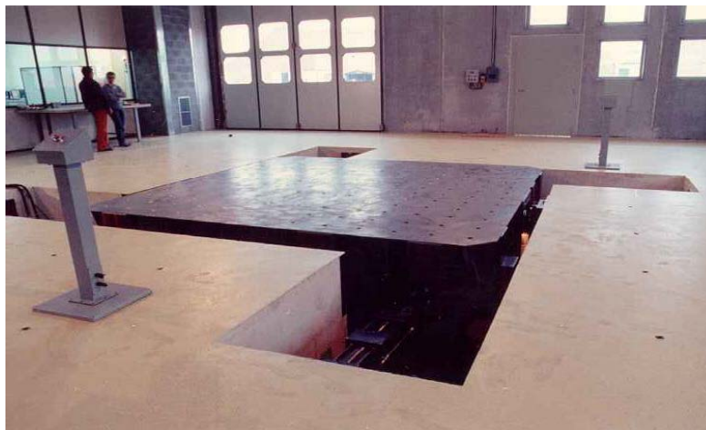
Figure 18: The 6-DOF MASTER Shaking Table at Enel.Hydro/ISMES Premises (Seriate, BG, Italy)
